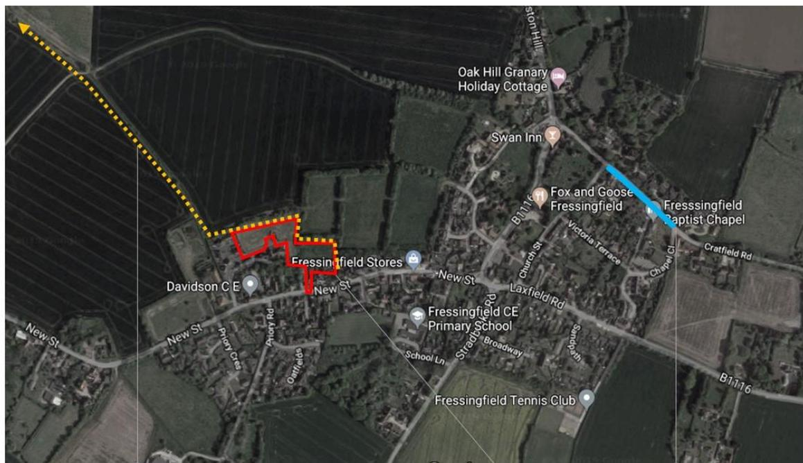
Proposed route attenuated surface water flows from site would take via existing ditch network. Ditch network discharges to small stream which flows north-east away from village
